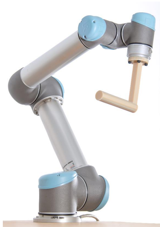
Figure 14. Universal robot with 3D printed probe for leak tests
