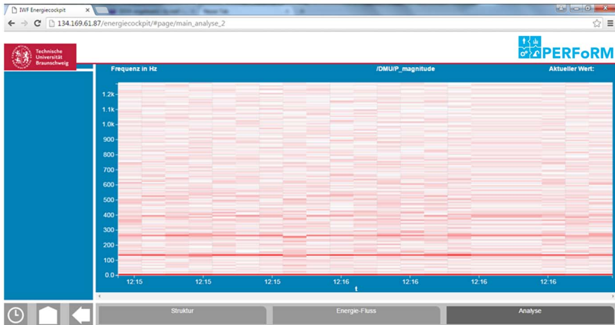
Figure 11: Universal Web-based Visualisation: Exemplary view of a fast Fourier transformation on a power signature
