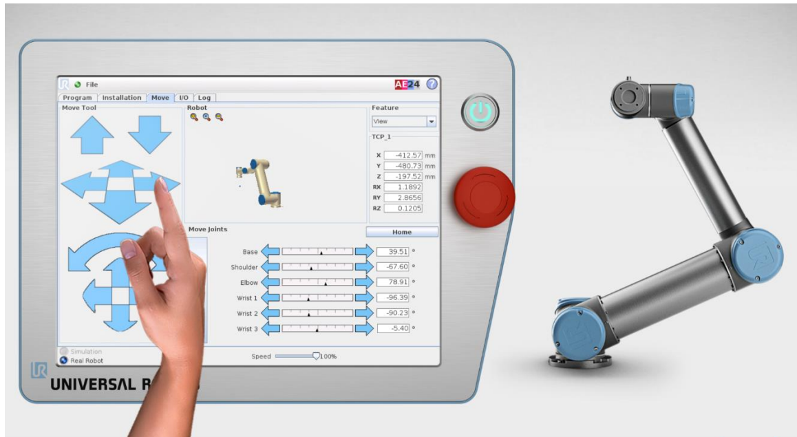
Figure 17 The teach pendant command to move robot
