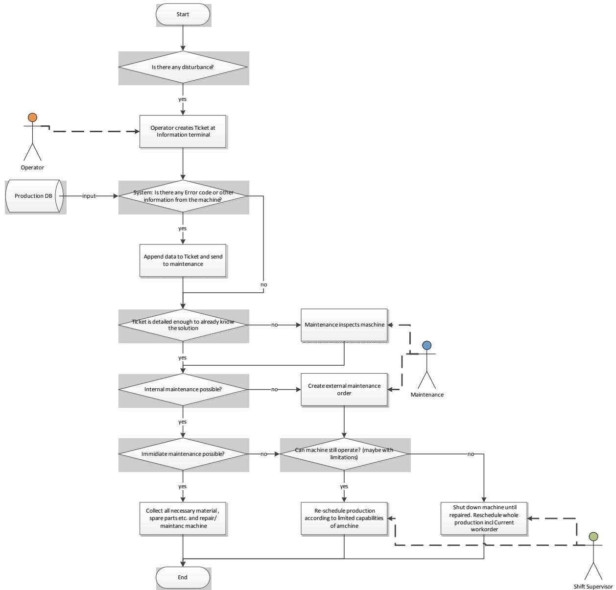
Figure 7: simplified Flow Chart for Disturbance reaction
