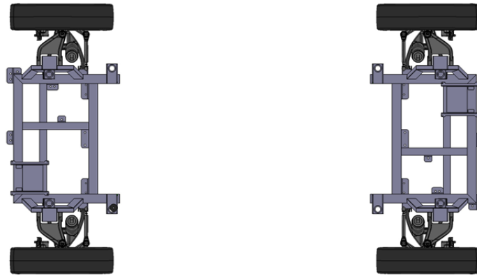
Figure 4 : Axle frame: Within the purpose of this project the axle frame is identical for both the front and the rear motorized axles and for both the passenger and the cargo configurations.
